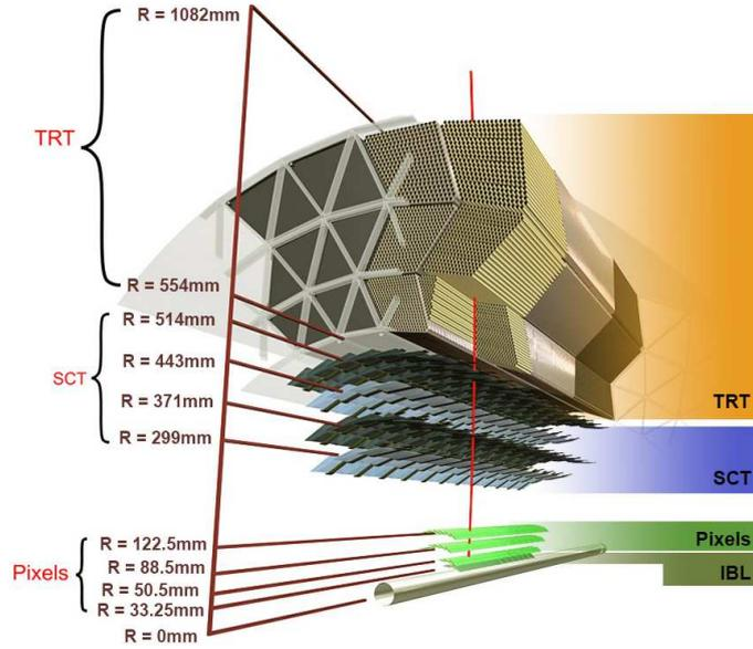
Figure 15: A cutaway view of the ATLAS inner detector [30].
