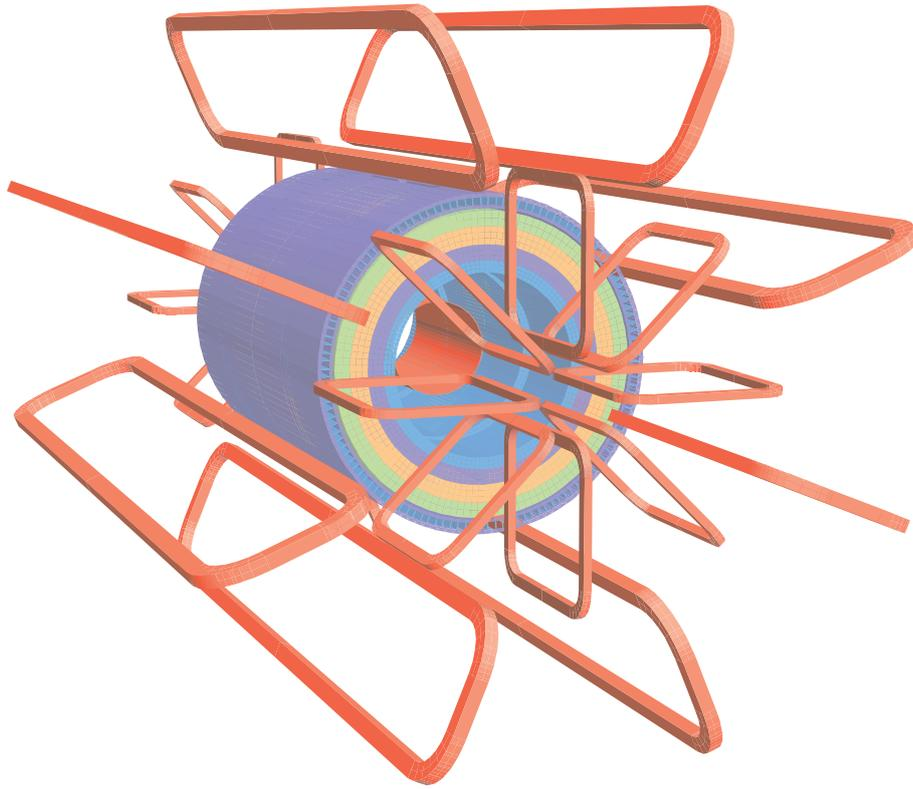
Figure 14: A cutaway view of the ATLAS superconducting magnetic system.
