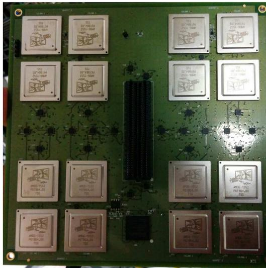
Figure 54: A photo of a LAMB board with 16 AM chips mounted.
