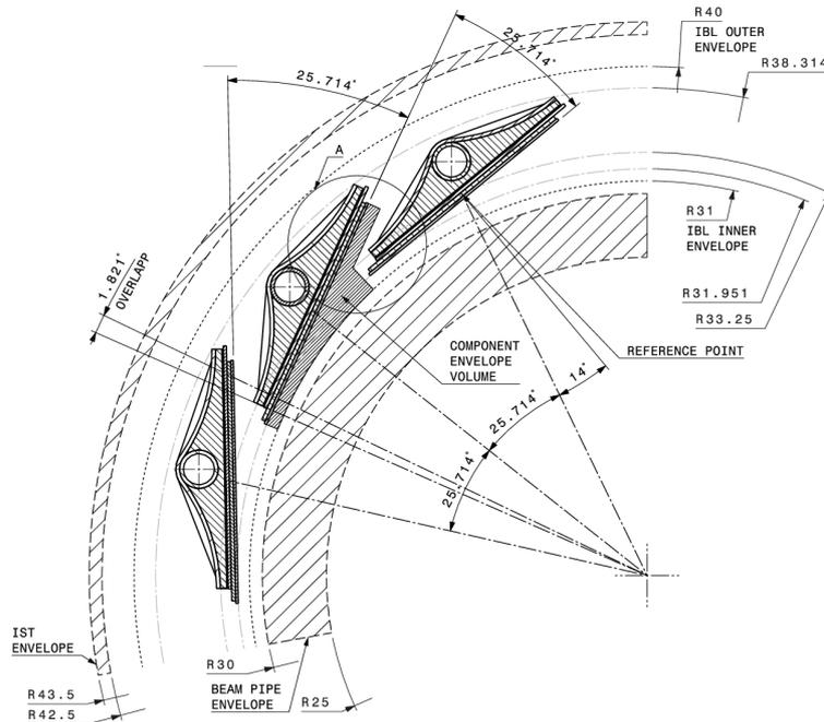
Figure 17: A schematic view of the IBL structure in  $r - \phi$  plane.
