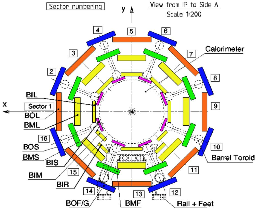
Figure 31: A schematic  $R - \phi$  view of the ATLAS Muon Spectrometer along with other sub-detectors.
