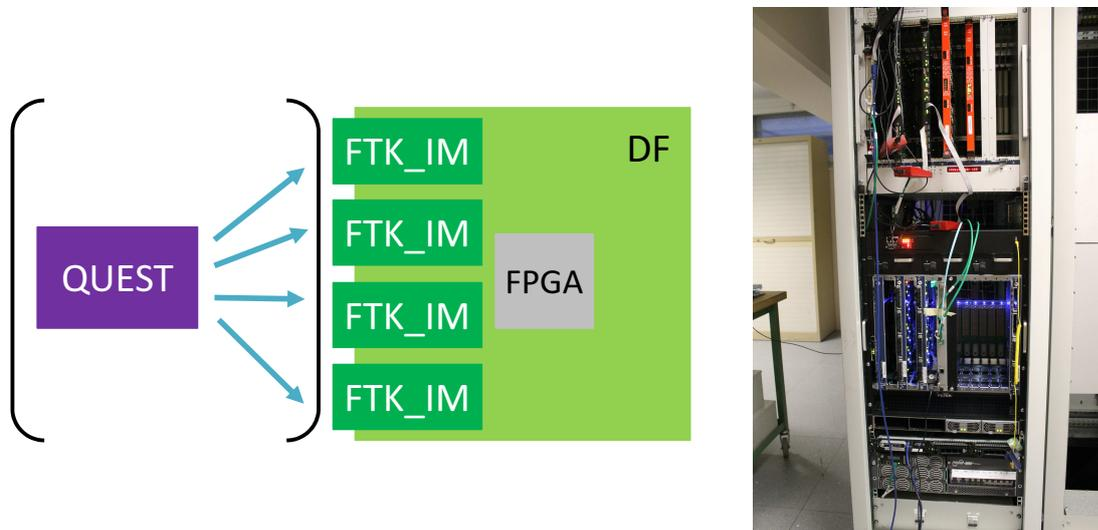
Figure 94: A schematic view and photo of the test stand setup built at the CERN. Boards in the lower rack are the DFs and in the upper rack are the AMBs and the SSBs in the photo. The AMBs have red front panel, while the SSBs have black front panel. The AUX cards are installed behind the AMBs.
