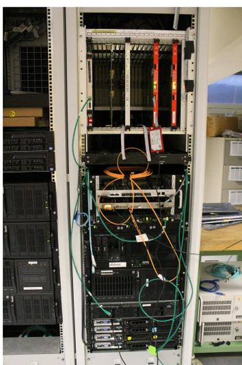
Figure 95: A photo of test setup of the FLIC crate. The FLIC can be seen in the middle crate. The rack is placed at the next of the one of Fig. 94.
