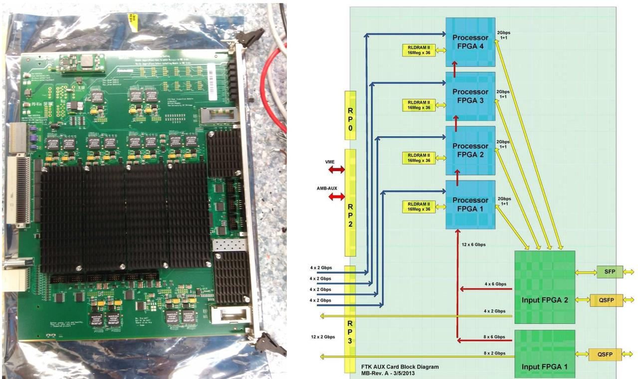
Figure 52: A photo (left) and functional overview (right) of the AUX.
