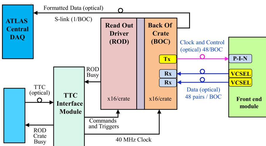
Figure 20: A schematic diagram of the SCT data acquisition.
