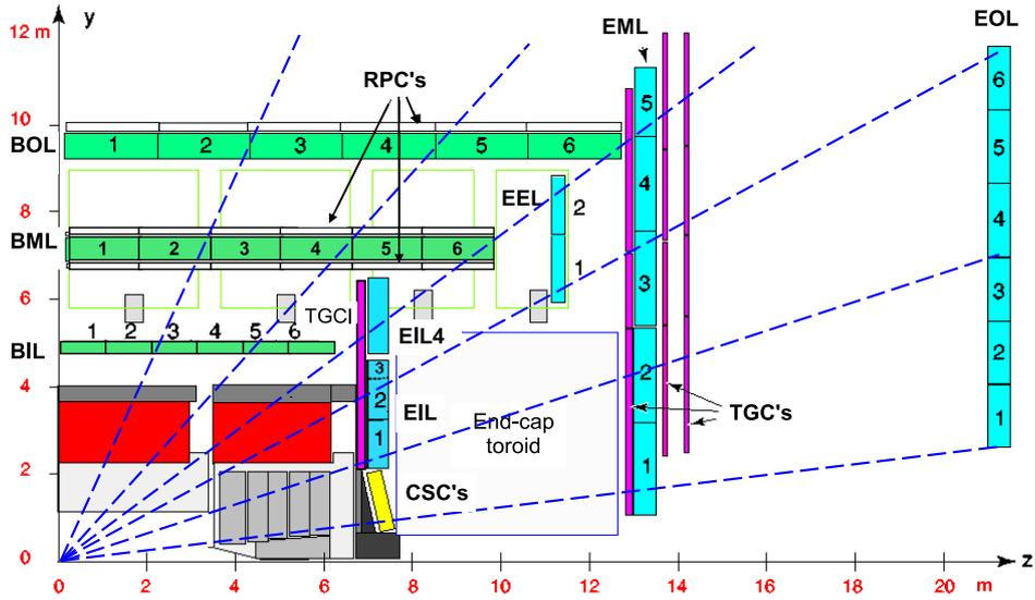
Figure 30: A schematic  $R - Z$  view of the ATLAS Muon Spectrometer.
