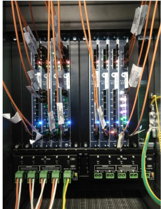
Figure 97: Photos of the DFs and IMs installed in an ATCA crate (left) and the RTMs on its back plane (right).
