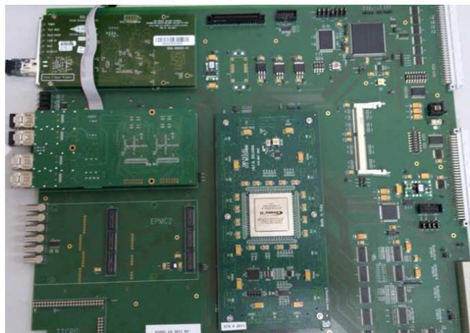
Figure 78: A photo of the EDRO board with one IM and HOLA mounted. The top most card is HOLA and the next one is an IM. The mezzanine mounted at the center holds Stratix II FPGA.
