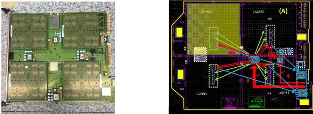
Figure 53: A photo of an AMB with 4 LAMBs mounted (left) and a schematic overview of the data flow in an AMB (right).
