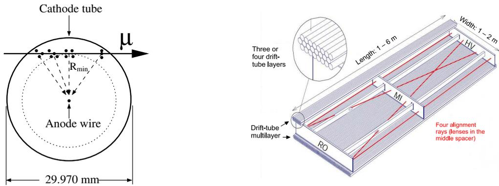
Figure 32: (left) Cross-section of a MDT tube. (right) Mechanical structure of a MDT chamber.
