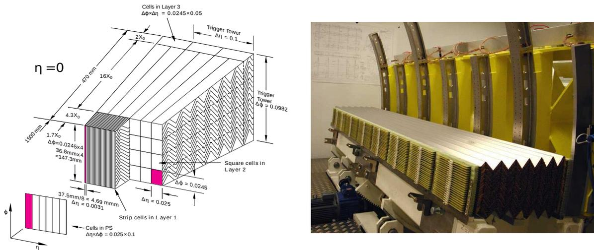
Figure 25: (left) A sketch of a barrel module of the Electro-Magnetic calorimeter. (right) A photo of a partly stacked modules of the barrel Electro-Magnetic Calorimeter.
