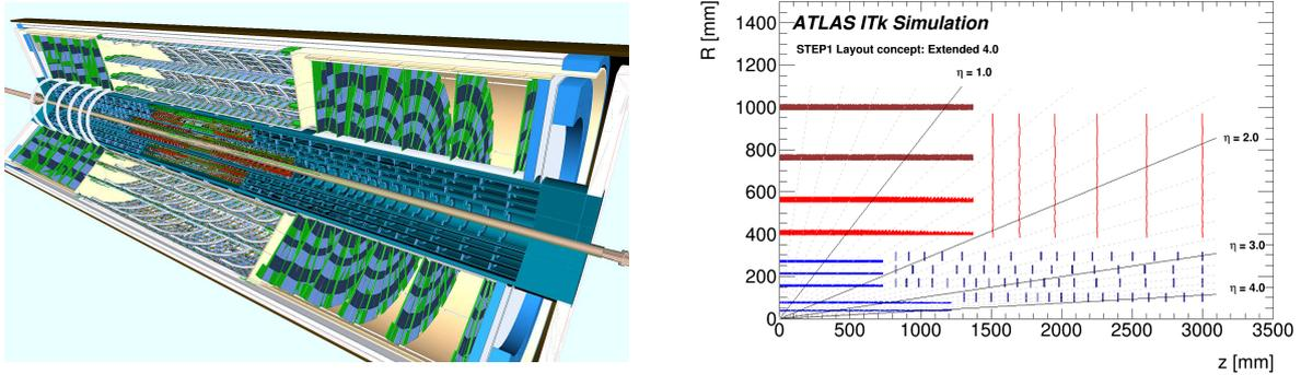
Figure 106: A visualization of the ITk in simulation (left) and one of the options of the planned ITk layout (right). In the layout, the blue ones represent pixel detectors and the red ones represent strip detectors.
