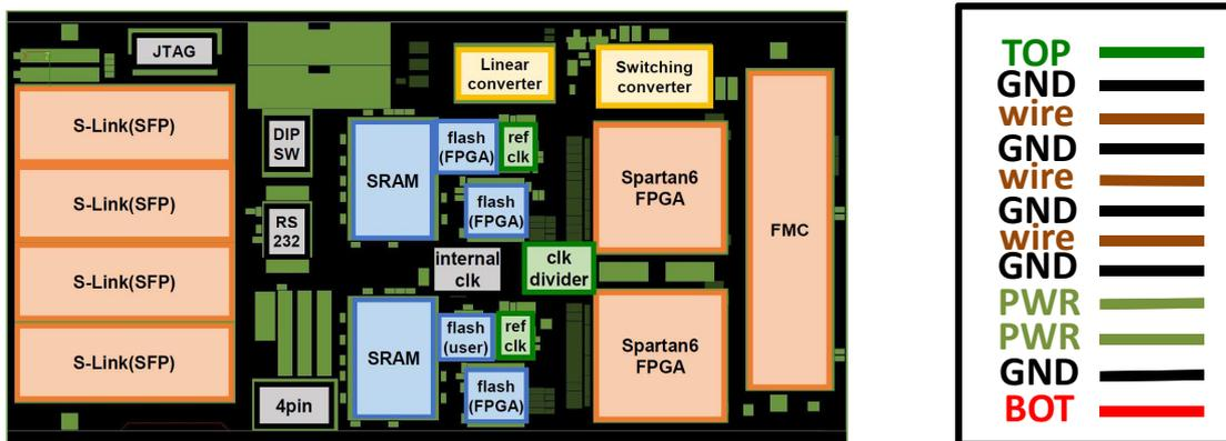
Figure 84: Final components of the IM board are shown in the left and the IM board structure of 12 layer is shown in the right. TOP and BOT stand for top layer and bottom layer, GND for ground layer, wire for the layer which lines is running, and the PWR is the layer used for power supply lines.
