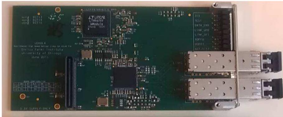
Figure 46: A photo of the dual-output HOLA.
