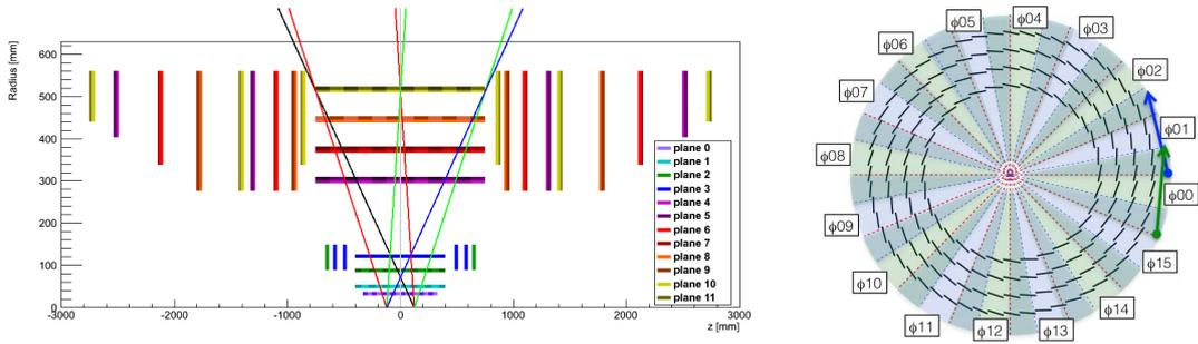
Figure 40: A schematic view of the detector segmentation for the FTK processing.  $\eta$  is segmented into 4 regions and  $\phi$  is into 16 regions. The FTK algorithms run in parallel with these 64 regions.
