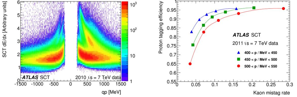
Figure 23: (left) Energy loss measured in the SCT as a function of momentum multiplied by charge. Protons are enhanced in the sample by collecting particles originated from secondary interaction with detector materials. (right) Proton tagging efficiency as a function of kaon mistag rate.
