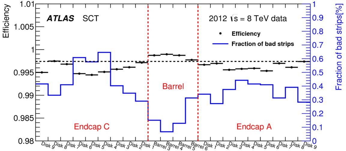
Figure 22: Mean intrinsic efficiency for each layer of the SCT.
