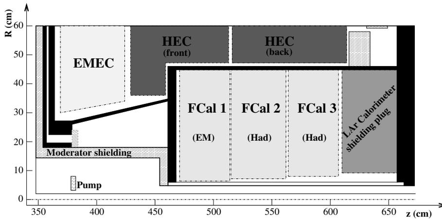
Figure 28: A schematic diagram of the three FCal modules located in the endcap.
