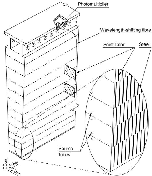
Figure 26: A schematic view of the mechanical assembly and the optical readout of the tile calorimeter.
