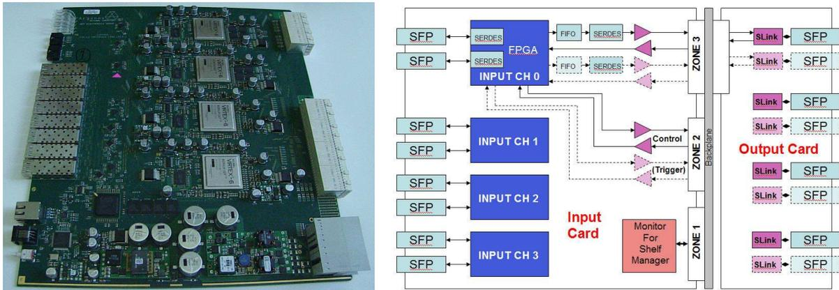
Figure 59: A photo of the FLIC (left) and a functional overview of the FLIC (right).
