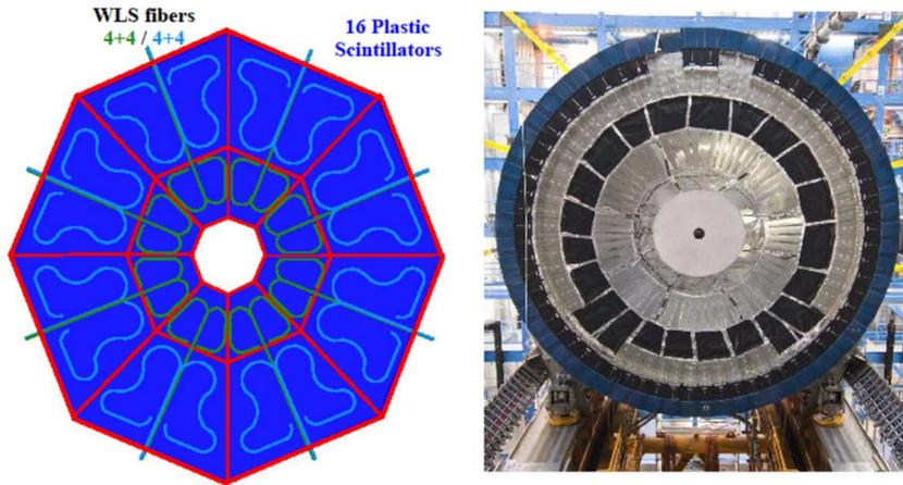
Figure 34: A schematic view and a photo of the Minimum Bias Trigger Scintillator [50].
