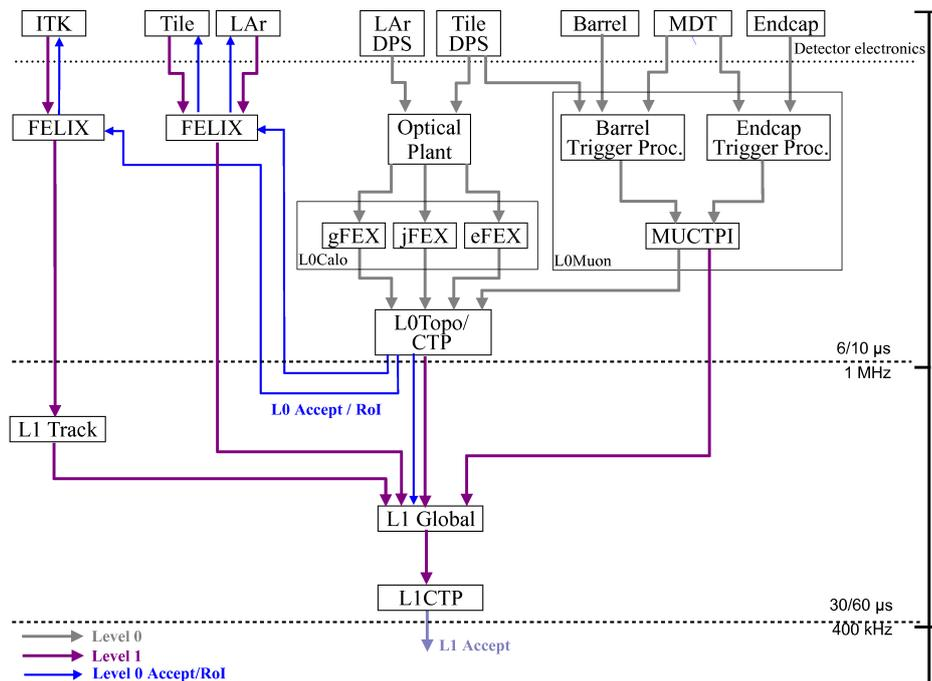
Figure 107: A schematic view of the ATLAS L0 and L1 trigger system planned at the HL-LHC.
