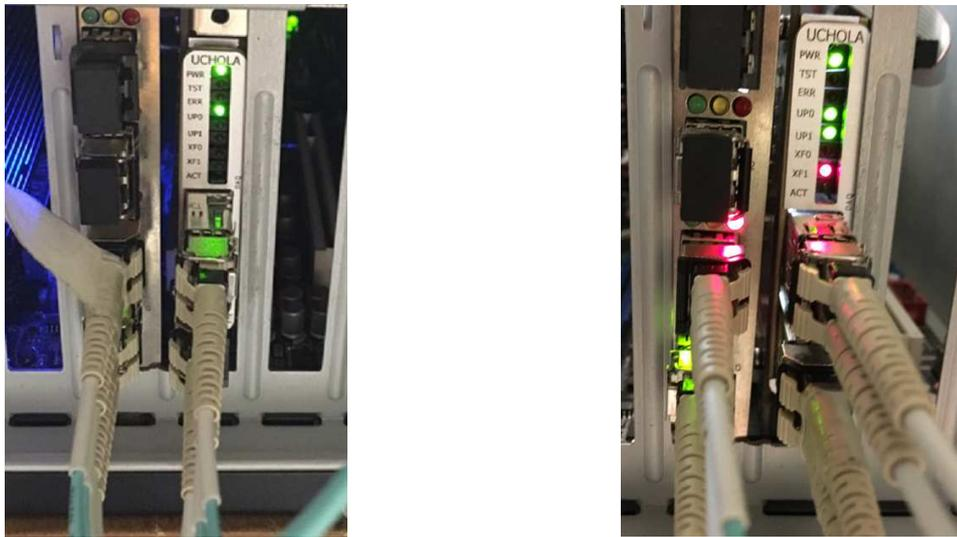
Figure 100: Photos of the front view of the FILAR (left card in each photo) and the D-HOLA (right card in each photo). The fiber connected to upper channel of the D-HOLA goes to the FILAR, and the other goes to the IM. The LEDs stands for POWER ON, Test, Error, Link up for main channel, Link up for the FTK channel, XOFF from main channel, XOFF from the FTK channel, action from the top to bottom.
