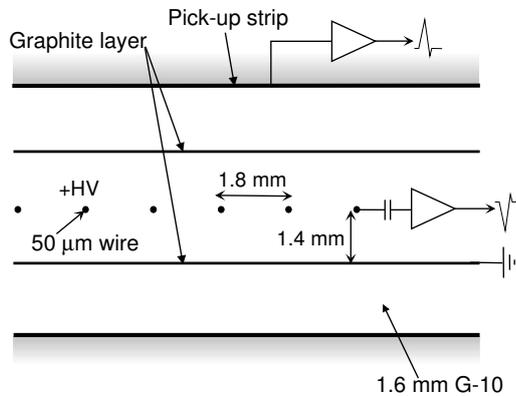
Figure 33: A schematic view of the TGC structure.
