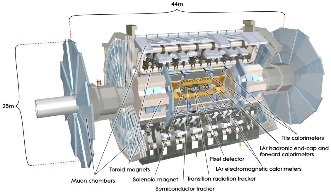
Figure 12: A cutaway view of the ATLAS detector.
