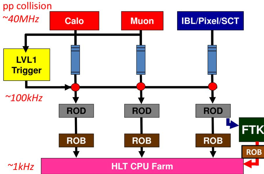
Figure 1: An overview of current ATLAS trigger system with the FTK.
