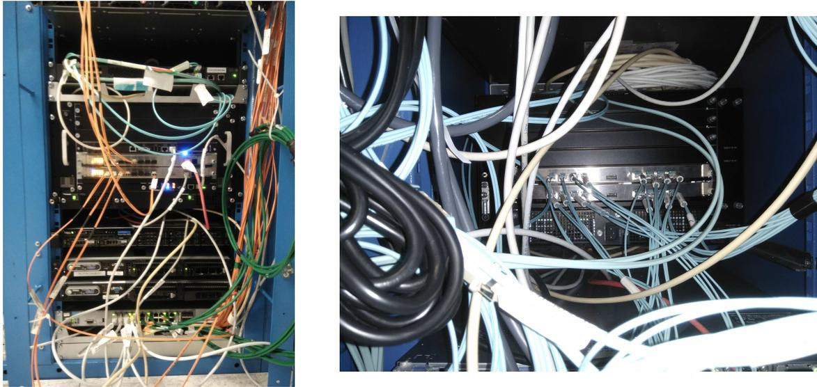
Figure 99: Photos of the FLIC cards installed in one of the VME racks (left) and the RTMs on its back plane (right).
