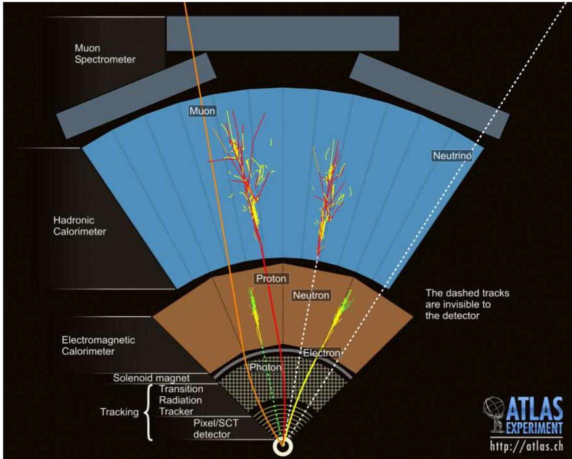
Figure 13: A schematic view of particle detection in the ATLAS detector ensemble.
