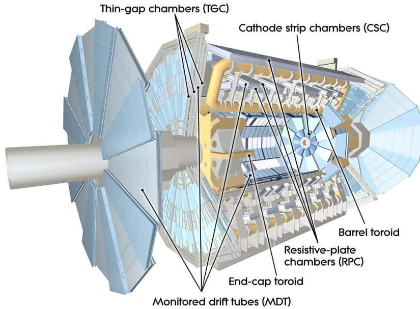
Figure 29: A cutaway view of the ATLAS Muon Spectrometers.
