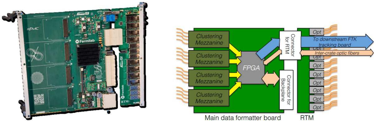
Figure 50: A photo (left) and a functional view (right) of the DF and its RTM.
