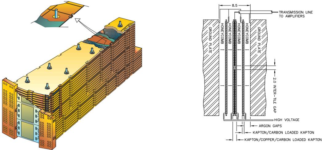
Figure 27: (left) A schematic view of a HEC module with the readout structure and the active-pad. (right) A schematic view of a HEC readout structure. All dimensions are shown in mm.
