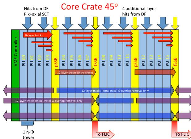
Figure 58: The SSBs in a core crate and data flow in and out of the SSBs.
