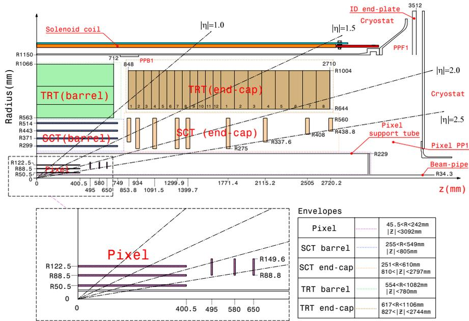
Figure 16: A detailed configuration of the ATLAS inner detectors.
