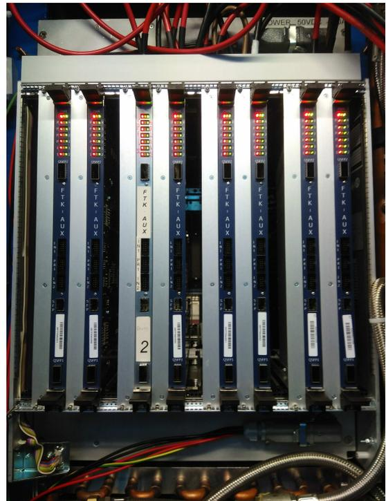
Figure 98: Photos of the AMBs and SSBs installed in a VME rack (left) and the AUX cards on its back plane (right).
