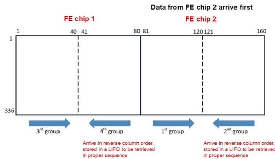
Figure 48: A schematic view of the readout order of FE chips of the IBL planar module.
