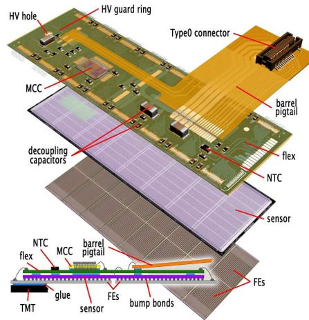
Figure 18: A schematic view of the pixel modules.
