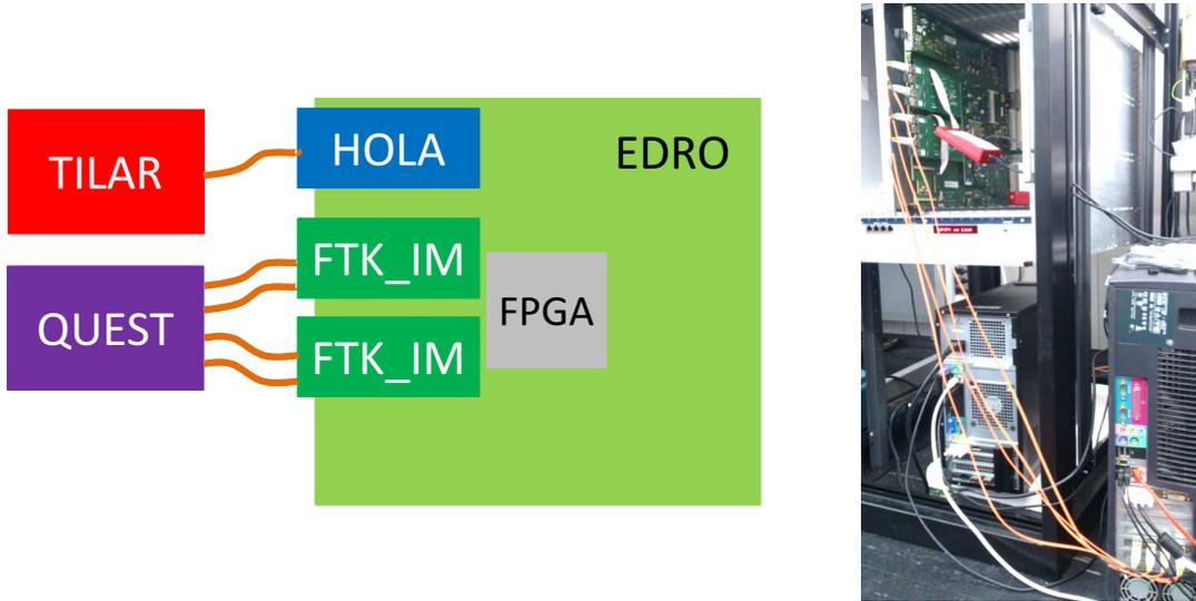
Figure 80: A schematic view (left) and photo (right) of the test bench built at Waseda. An EDRO board which holds two IMs and one HOLA card is in VME rack. The TILAR card is implemented on the computer under the VME rack, and the QUEST card is implemented on the right PC.
