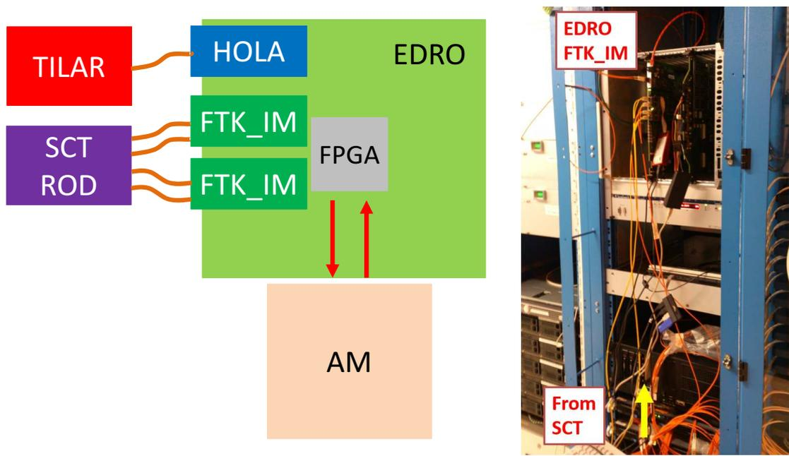
Figure 88: A schematic view and photo of the setup for the Vertical Slice test.
