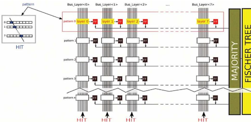
Figure 55: A schematic view of the AM chip array.
