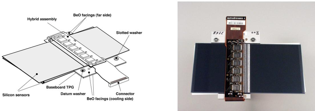
Figure 19: A schematic view and a picture of a SCT module.
