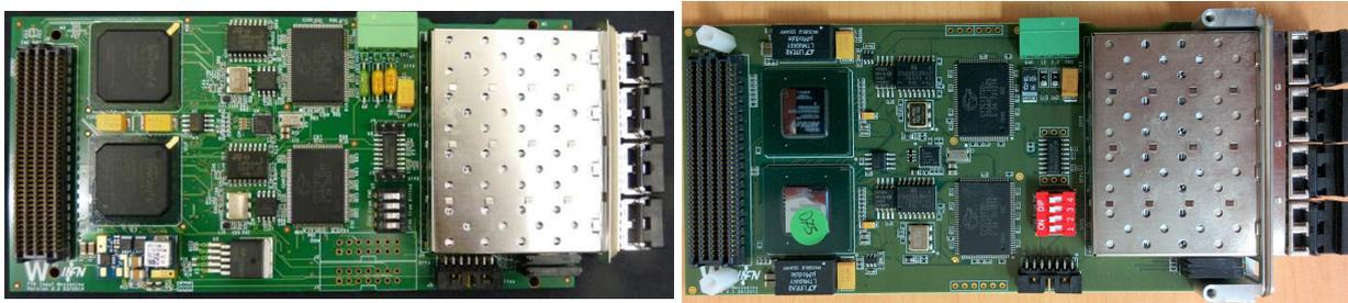
Figure 47: Photos of the IM with Spartan-6 FPGA (left) and Artix-7 FPGA (right).
