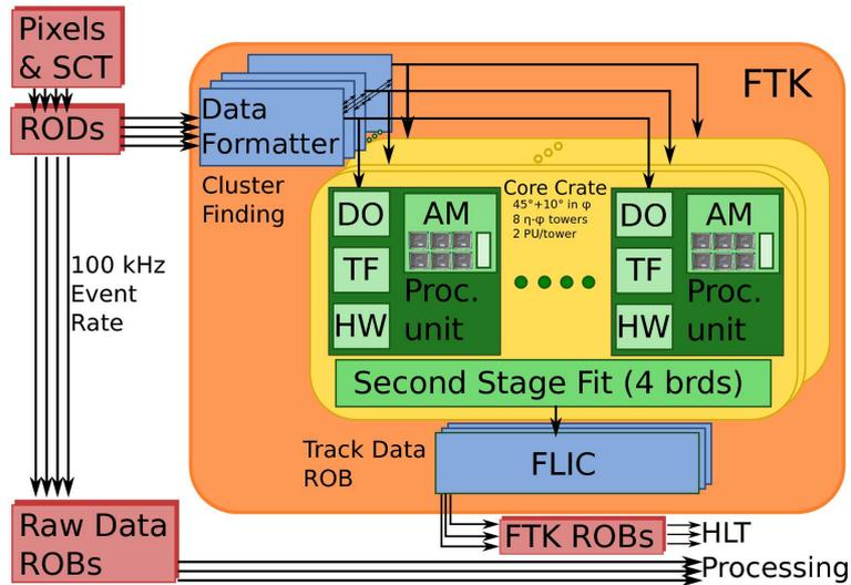
Figure 45: Functional overview of the FTK system.
