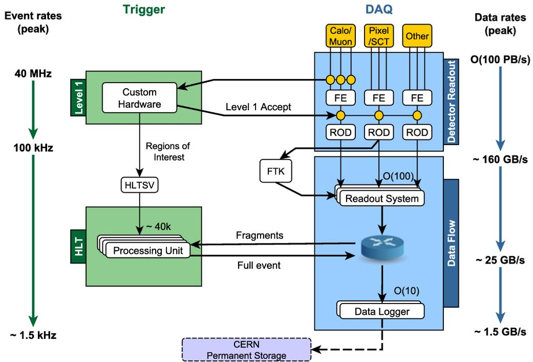
Figure 35: Functional diagram of the ATLAS Trigger and Data Acquisition system at LHC Run2.
