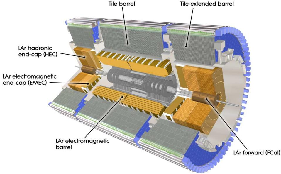
Figure 24: A cutaway view of the ATLAS Calorimeters.
