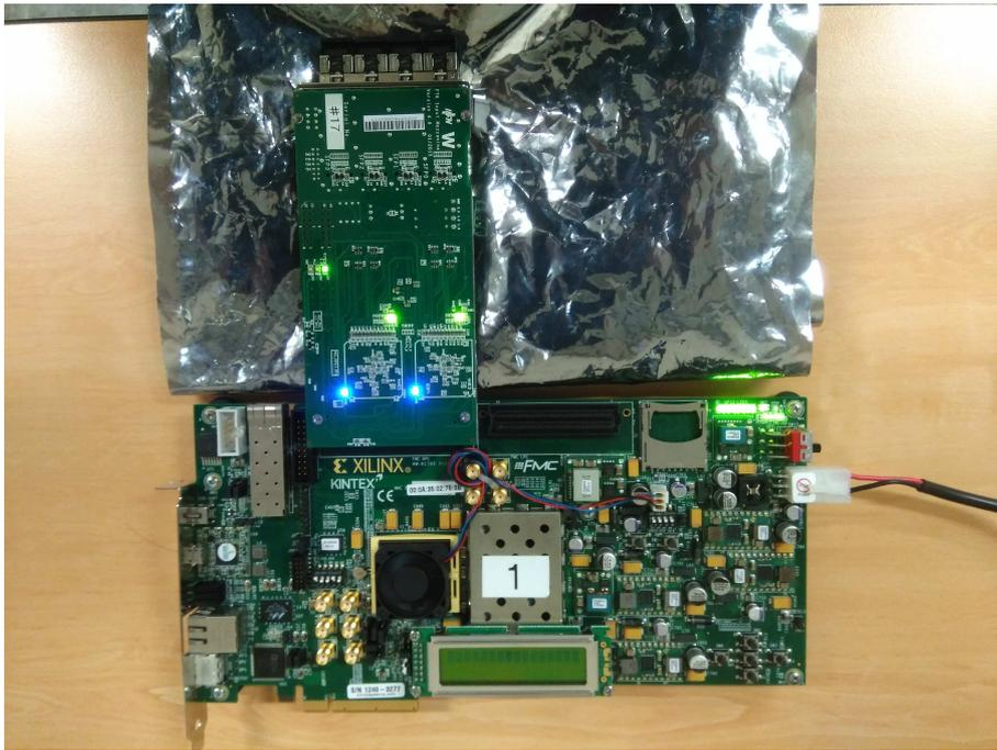
Figure 90: A photo of the KC705 with an IM mounted .
